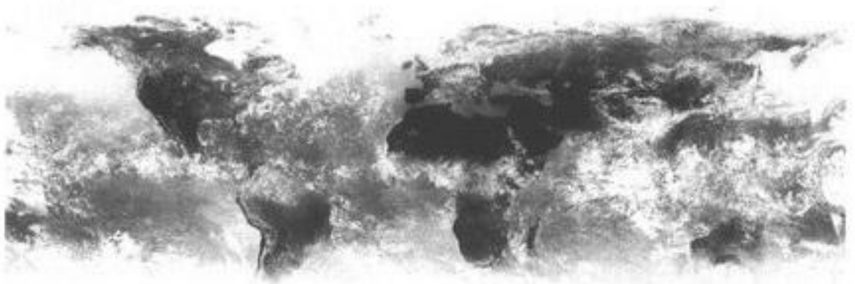
Figure 8. Weekly composite NDVI for 10–16 July 1989 with and without cloud mask (MASCI-generated overlay in white). The corresponding T_4 image is shown in Figure 7.
