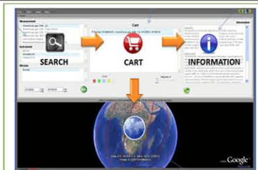
IMAGE B - The COVE User Interface is divided into 4 sections: Dynamic search menus, cart for selected missions, context-specific information panel, and Google Earth Viewport.
