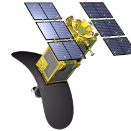
LOTUSat-1 (570 kg) with radar payload
