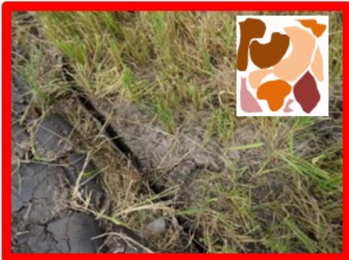
Unsaturated shrinking soil causing soil water suction
