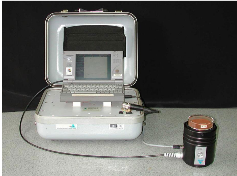
ASD Field Spec VNIR with optical setup
